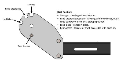
Note: In rear access position, Black Bar will not lock into place. Not for transporting.
